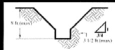
UNSUPPORTED VERTICALLY SIDED LOWER PORTION TYPE A SOIL 8 ft. or less in depth maximum vertical side of 3-1/2 ft
