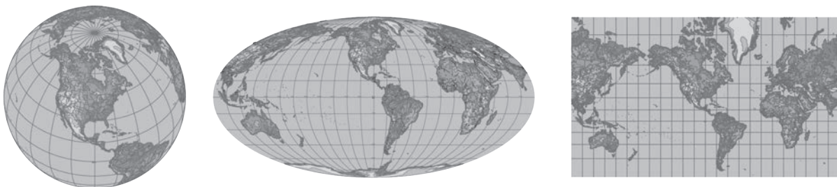
Figure 9. Map projections; three diagrams showing how a globe is transformed into a flat map.
